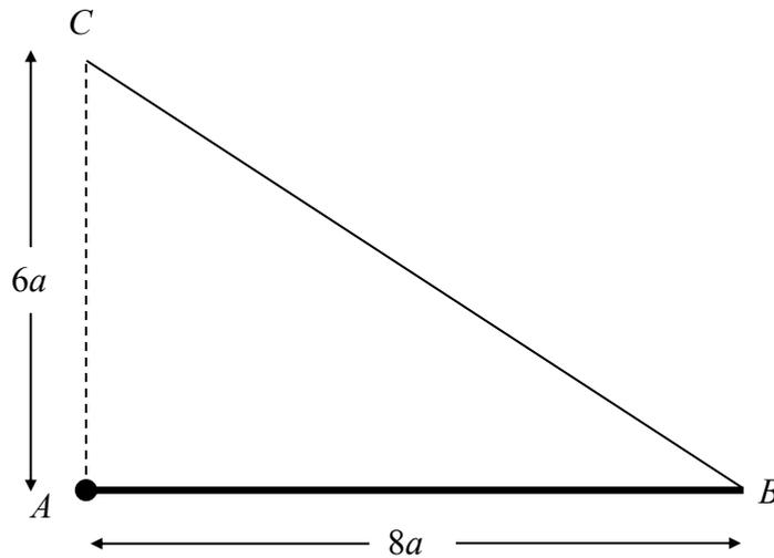
A uniform rod  $AB$ , of length  $8a$  and weight  $W$ , is free to rotate in a vertical plane about a smooth pivot at  $A$ . One end of a light inextensible string is attached to  $B$ . The other end is attached to point  $C$  which is vertically above  $A$ , with  $AC = 6a$ . The rod is in equilibrium with  $AB$  horizontal, as shown in Figure 1.
