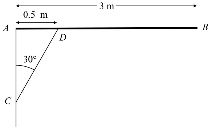
A uniform pole  $AB$ , of mass 30 kg and length 3 m, is smoothly hinged to a vertical wall at one end  $A$ . The pole is held in equilibrium in a horizontal position by a light rod  $CD$ . One end  $C$  of the rod is fixed to the wall vertically below  $A$ . The other end  $D$  is freely jointed to the pole so that  $\angle ACD = 30^\circ$  and  $AD = 0.5$  m, as shown in Figure 2. Find
