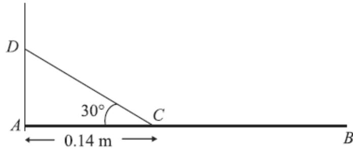
A uniform beam  $AB$  of mass  $2$  kg is freely hinged at one end  $A$  to a vertical wall. The beam is held in equilibrium in a horizontal position by a rope which is attached to a point  $C$  on the beam, where  $AC = 0.14$  m. The rope is attached to the point  $D$  on the wall vertically above  $A$ , where  $\angle ACD = 30^\circ$ , as shown in Figure 3. The beam is modelled as a uniform rod and the rope as a light inextensible string. The tension in the rope is  $63$  N.
